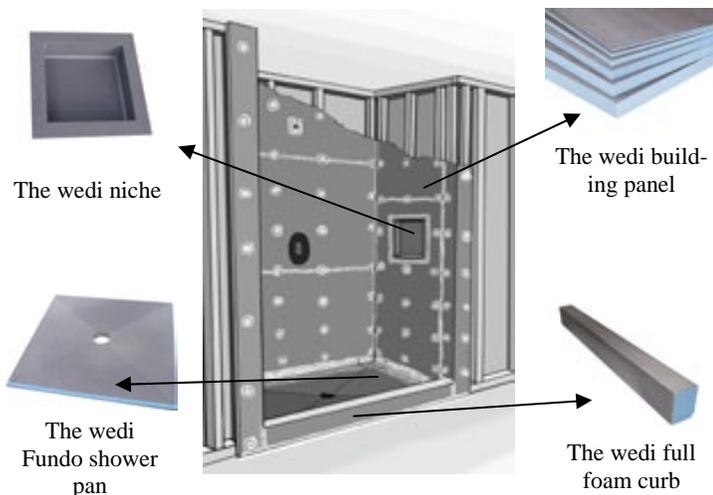
The Wedi systems save 80% of the weight that conventional systems add to the building structure and offer thermal insulation value behind the tile. Fundo shower pans are easily trimmed or extended to fit the available shower area. Wedi has also developed curbs, ramps, wall inserts and bench seats to be used in conjunction with the Wedi Shower System allowing them to offer the only complete tile-ready shower waterproofing system on the market.
